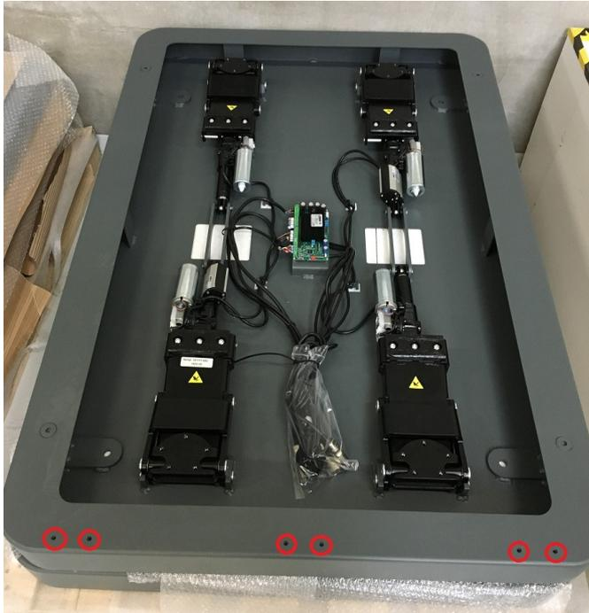
3.1. The side with the six screw holes (circled with red) must be placed at the front end of the robot.
