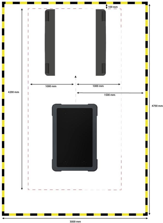
4.1. The floor around the pallet rack must be marked to indicate where the personnel protection means are muted. This can for example be done with signal tape.
