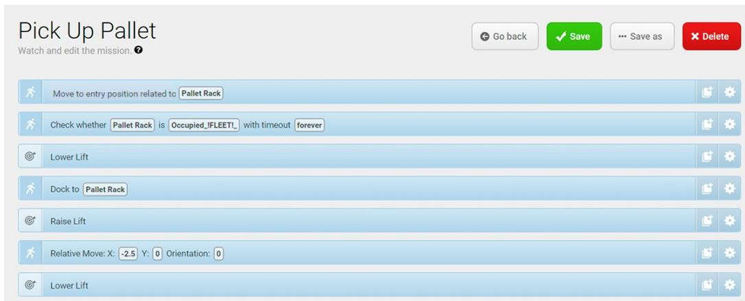
5.1. MiR1000 drives to the entry position in front of the MiR1000 Lift and checks if there is a pallet (check position status is optional). If there is a pallet, MiR1000 lowers the lift, docks to the pallet rack, lifts off the pallet, exits the pallet rack and lowers the lift again.
