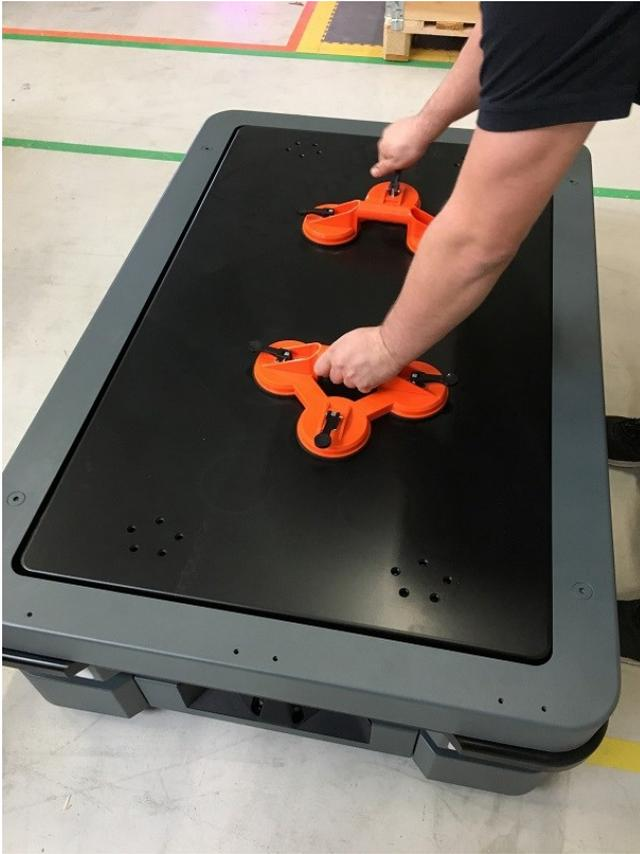
7. Screw in all twenty screws to fix the cover to the lifting device. Ensure the screws are plane with the lift cover.
